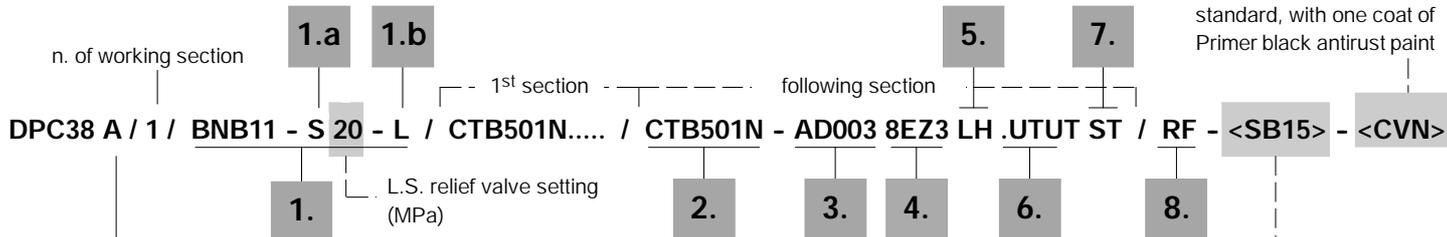
A = Directional valve for fixed displacement pump (open centre)
