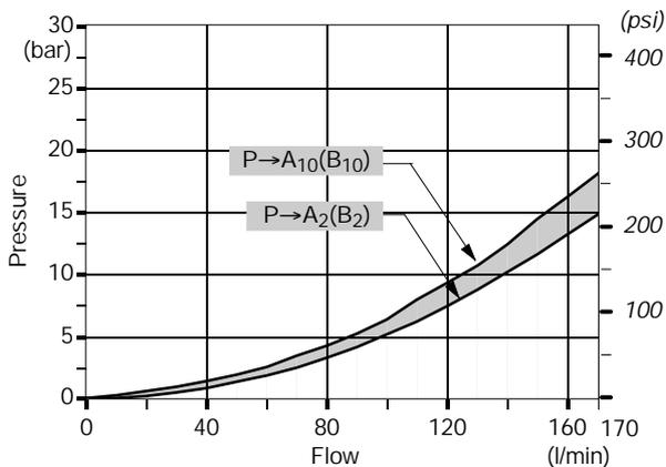
Working section with compensator
